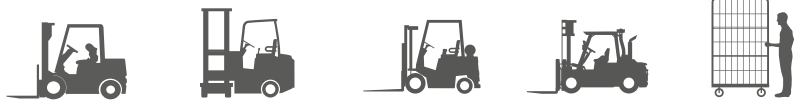
Lightweight counterbalance FLT Very narrow aisle FLT Heavy duty counterbalance FLT Engine counterbalance heavy duty FLT Frame roll container
