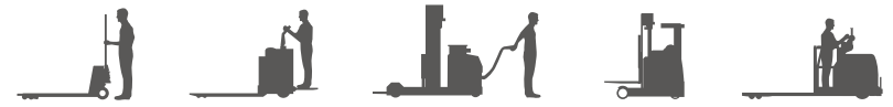
Manual pallet truck Electric pedestrian truck Electric pedestrian stacker Electric high reach truck Horizontal order picker
