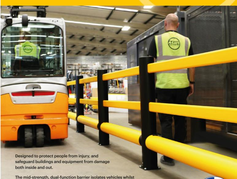
The mid-strength, dual-function barrier isolates vehicles whilst also guiding pedestrians. The traffic rail provides physical
