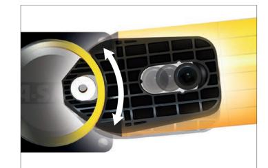
PHASE 2: Compression of the pocket continues to disperse energy as the coupling rotates around the post pin to activate further absorption.
